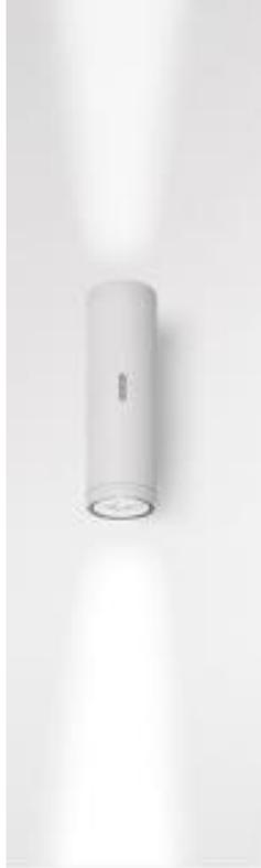
*Figure 15: The Calumet luminaire from Artemide is an example of a luminaire with a separate luminous top and bottom, which cannot be represented accurately with a single IES file model because the luminous area cannot be defined to represent 2 emitting surfaces separated by non-luminous sides. This luminaire should be represented by two separate photometric files, one for the uplight and one for the downlight. [Source: <https://www.artemide.com/en/products/outdoor#> (11/26/18)]*
