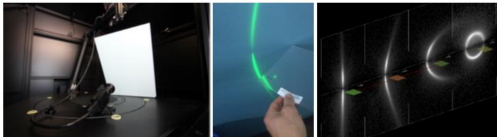
Figure 2: These images show the camera & screen in our HDR imaging based BSDF measurement device, a laser directed through an anisotropic linear diffuser from Bright View Technologies from about 30° off-axis from the micro-prismatic features, and the simulated light scattering properties from 4 different material orientations with respect to the incoming light direction. The image showing the green laser directed through the material has a similar material orientation as the 2nd simulated orientation in the image on the right.
