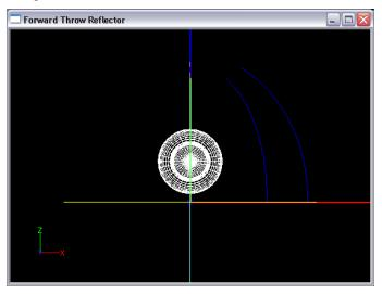
You can see from this view that changing the start point of V3 had a secondary effect of making it taller. The height of the profiles is based on a reflector extent angle rather than a fixed height, so we will need to adjust this angle to bring V3 back to the same height as V1 and V2.
