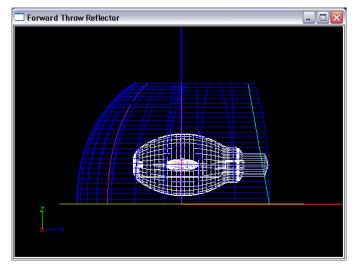
32. Linking the front reflector to the main reflector will make the position of the front reflector adjust automatically when we make changes to the main reflector. Select the front reflector and under Start & Extent in the property control change the Start Linkage from None to H1.
