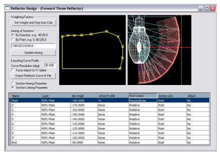
25. In the Start row, click on the Prof Orient value to change it from *Relative* to *Perpendicular*, so that the V1 profile is perpendicular to each H1 section that V1 is linked to.
