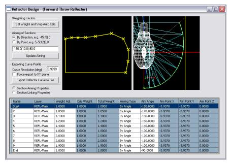
11. Next, since the reflector will be segmented, we need to make sure that H1 will take this into account. Keep H1 selected and find the Curve Resolution under **Section/Profile** in the middle of
