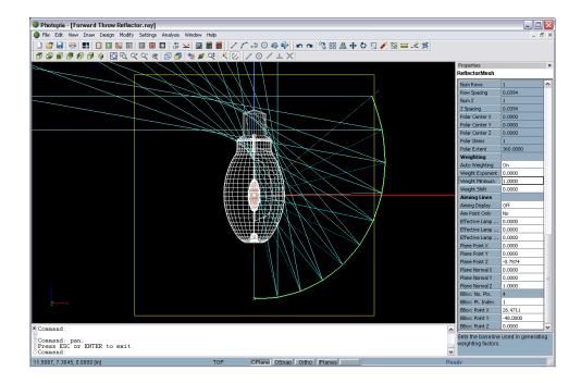
Now that the weighting is more evenly distributed, we can work from this baseline to create a weighting scheme that is more fitting to the application. To make a rectangle distribution of a Type III pattern, we will probably want more light aimed at the corners and sides of the light pattern than at the front. So we can change the weighting of H1 accordingly.
