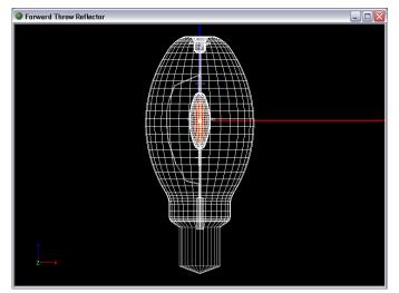
3. Once the lamp is inserted, then select it in the CAD view and use the Rotate command to rotate the lamp 180° about 0,0.
