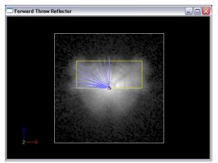
The corner light has filled in well, but there are still bright spots near the center of the light pattern. To continue working on this issue, we can adjust the weighting of the other vertical profiles as well.
