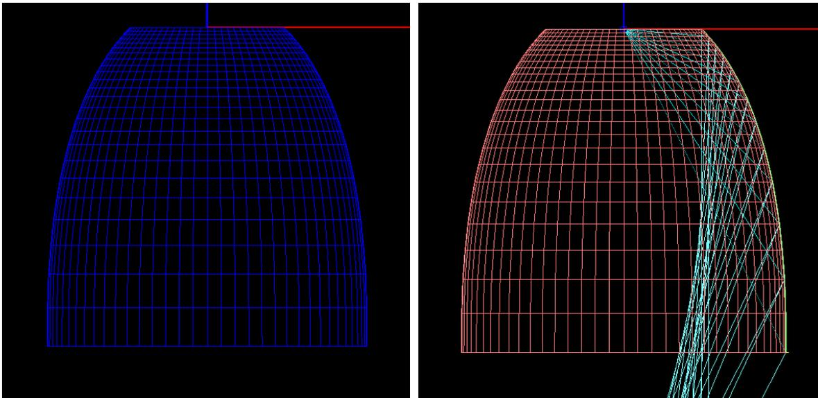
*The revolved reflector mesh. The 72 entered defined the number of segments around the circumference.*
