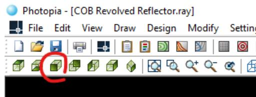
This will set the Construction Plane in line with the world XZ plane and put you in this view as well. This is the plane in which the profile should be created so the light will be directed toward world -Z axis, which is the 0° vertical angle in the intensity distribution.
